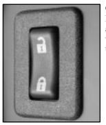
On the passenger side of the liftgate opening trim there is another power lock switch which can be used to lock or unlock all of the doors.
